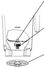
**Blade Agitator Assembly.** Blades are sharp; use caution when handling the blade. When inserting the blade assembly through the container bottom, align the flat sides. Gravity holds it in place while the retainer nut is tightened. Do not attempt to disassemble this part.
